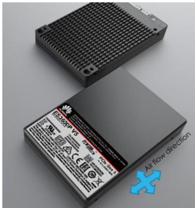
Figure 4-1 Design airflow direction
